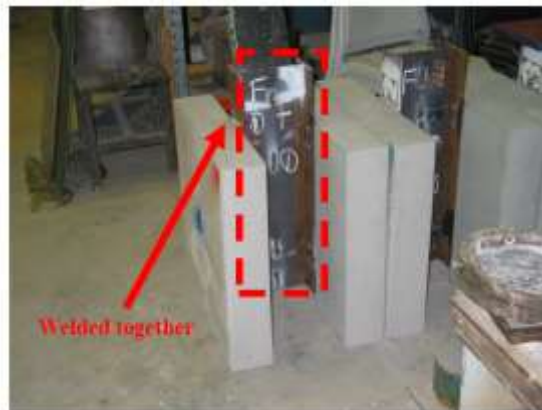
Figure.11 Push-out test specimens welded together
