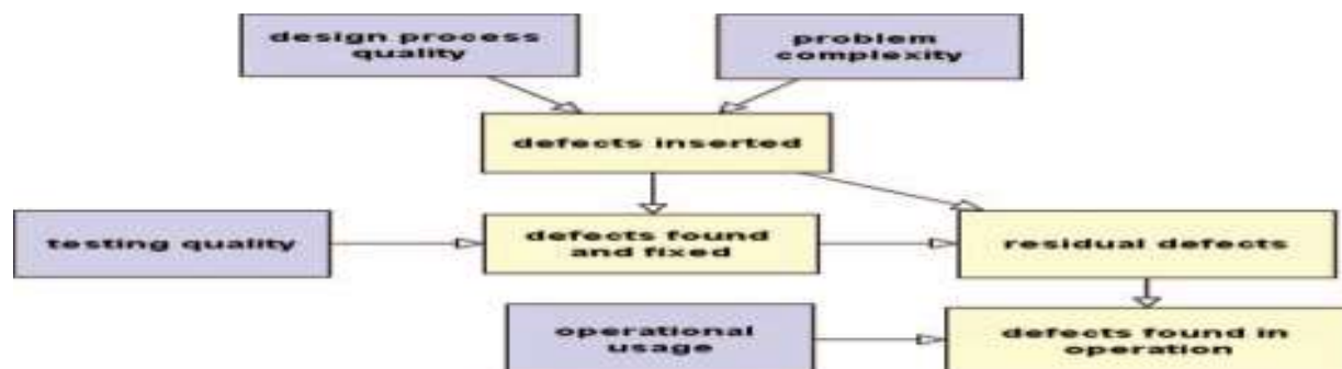
Fig. 1 Simplified version of a BN model for software reliability and defects prediction
