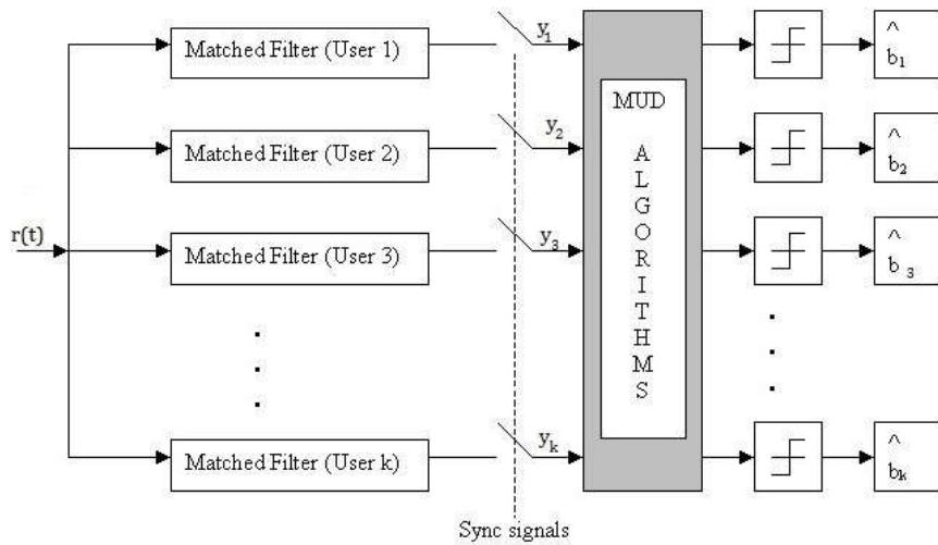
**Fig. 2 Multiuser detector for DS-CDMA system**
