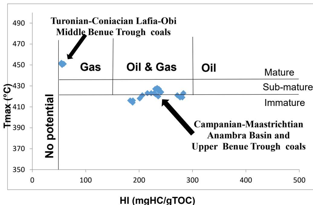
Fig. 5. HI-Tmax diagram for evaluating hydrocarbon proneness (after Obaje et al., 2004) shows that the organic matter are immature to sub-mature and overwhelmingly oil and gas-prone at deep-seated levels where appropriate maturities have been attained. Lafia-Obi deposits are entirely gas-prone.
