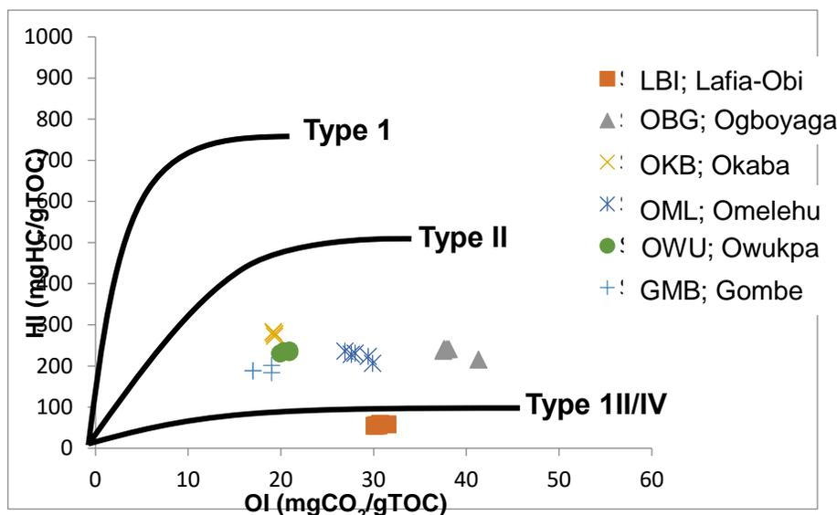
Fig. 4. Plots of Nigerian coal deposits on the Van Krevelen diagram showing that the deposits are overwhelmingly of Type II/Type III with potential to generate oil and gas except the Lafia-Obi coals that may have generated non-associated gas at deeper sections
