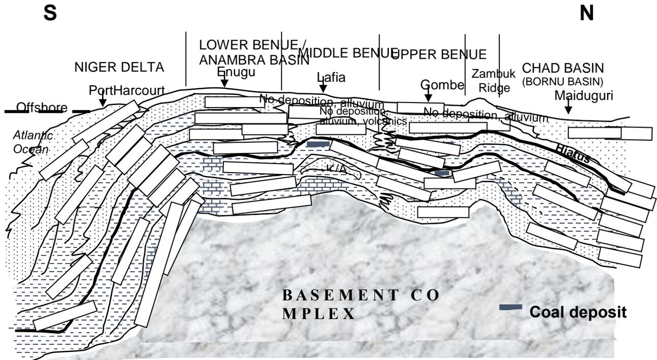
**Fig. 2. Stratigraphical cross-section from the Niger Delta through the Anambra Basin-Benue Trough onto the Chad Basin showing coal depositions within respective geological formations (after Obaje et al., 2004)**
