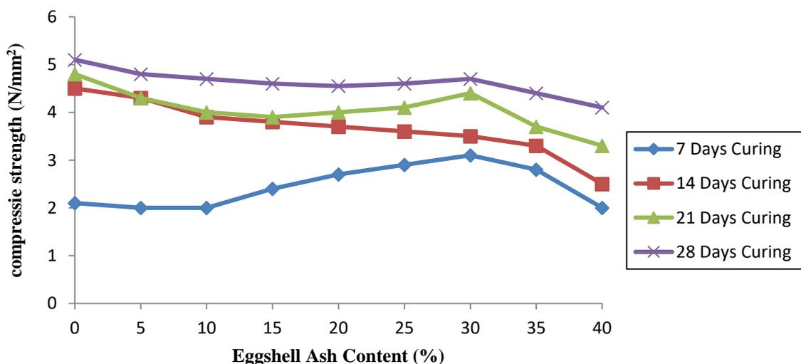
Figure 9: Variation of compressive strength of sandcrete block with eggshell ash content at varying curing period in days
