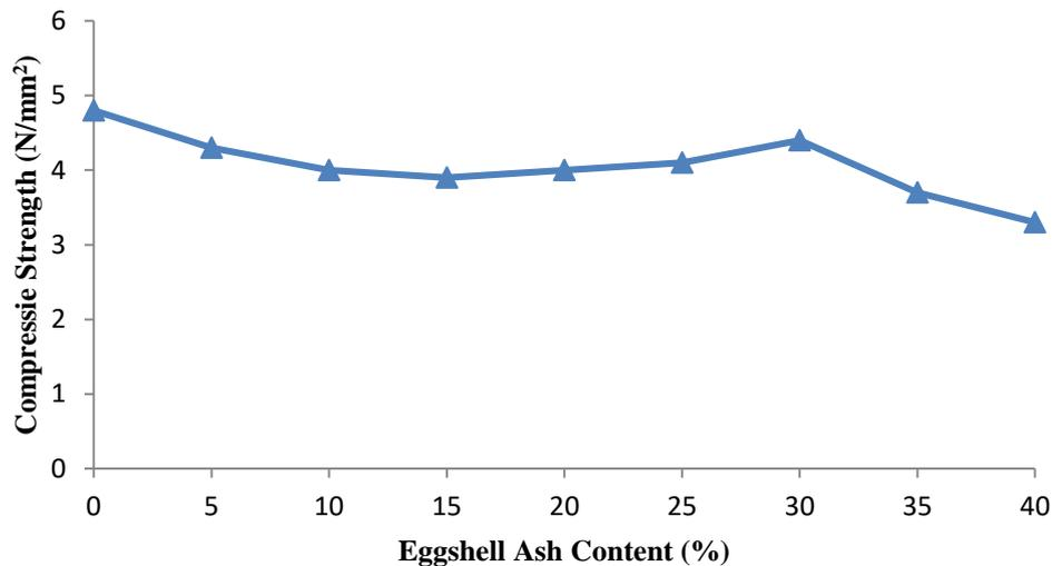
Figure 7: Variation of compressive strength of sandcrete block at varying eggshell ash content for 21 days curing period
