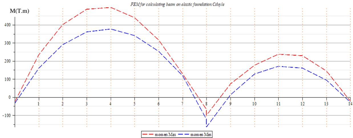
Figure 9. Interval moment graph in FEM.BEF
