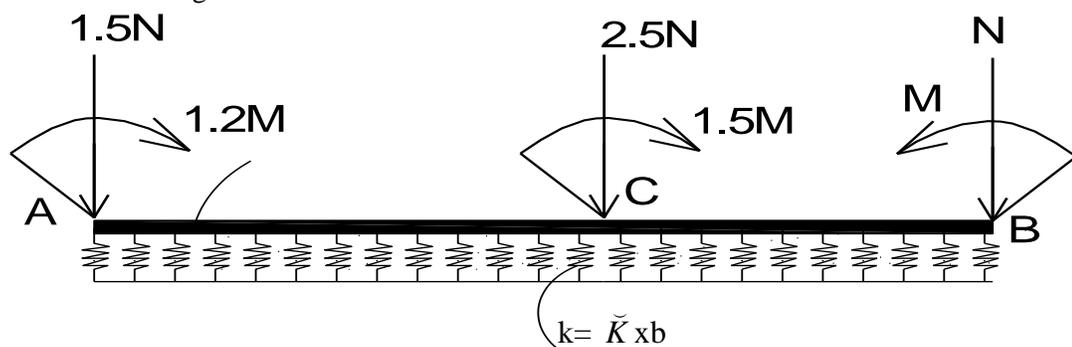
Fig. 8 Calculation model of beams on elastic foundation
