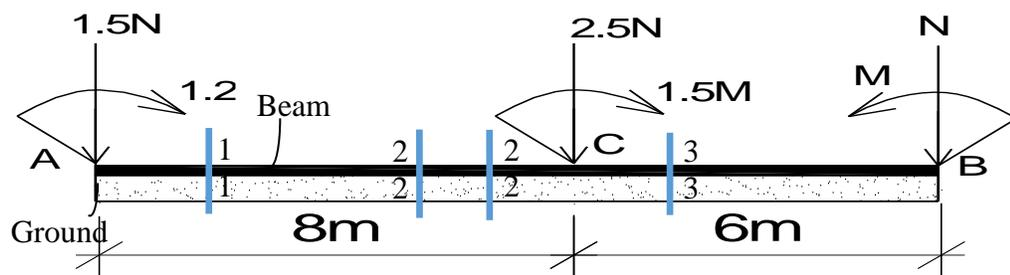
**Figure 7.** Structure diagram of foundation beam under load
