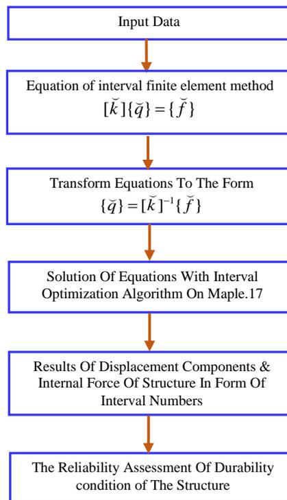
**Figure 6.** Block diagram of structural reliability assessment steps
