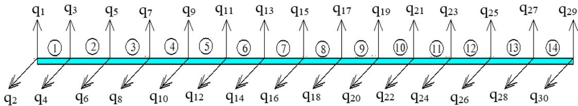
**Figure 8.** Element diagram of beam structure on elastic foundation
