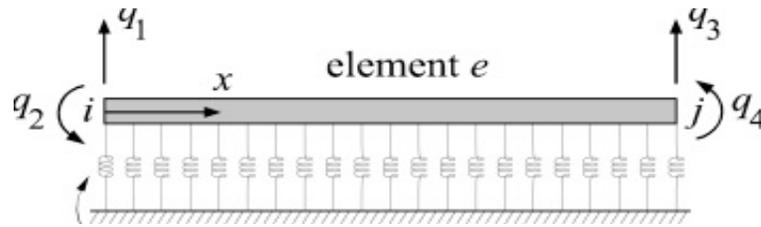
**Fig.1** Diagram of beam element on elastic foundation
