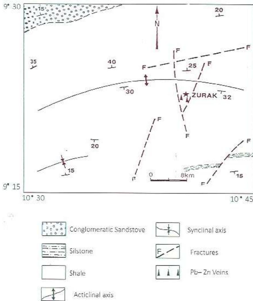
**Fig. 7: Geology and lead-zinc veins at Zurak (Mineral District Upper Benue) (Modified after Farrington 1952)**
