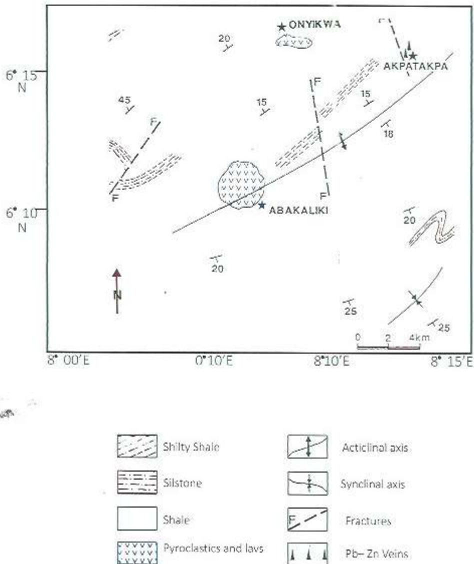
**Fig. 5: Geology and lead-zinc veins at Akpatakpa (Modified after Olade 1976)**
