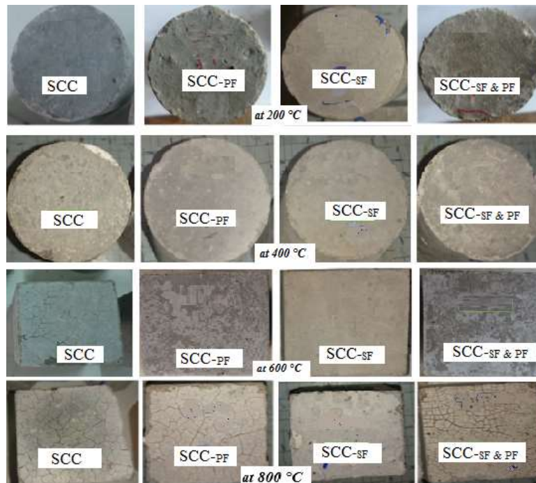
Figure 8. Surface behavior of SCC samples in 200, 400, 600 and 800 ° C with and without fibres
