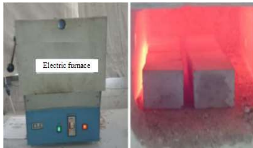
Figure 5: The electric oven used for heating the specimens
