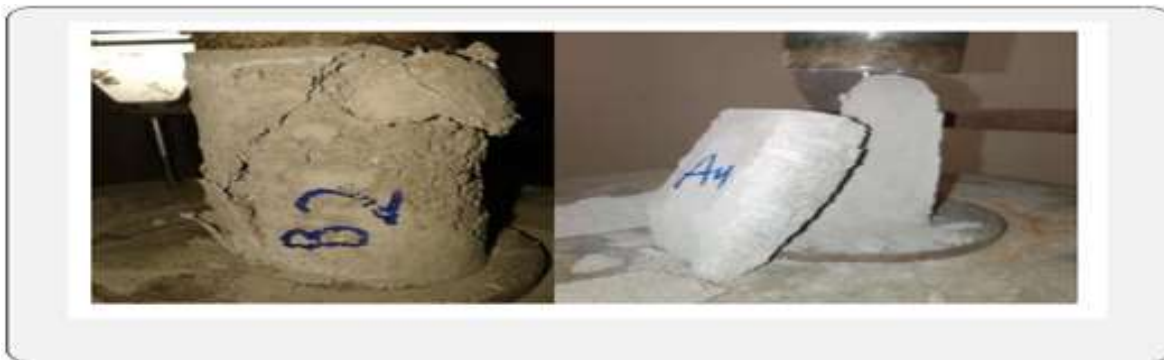
Figure 3: Typical shear failure of mixtures.
