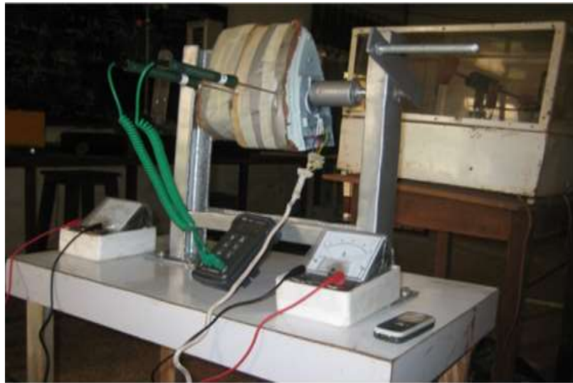
Plate 1. Photo of the experimental set up of modified lee disc apparatus
