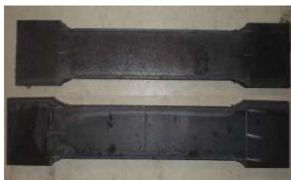
Fig 7.1 Sample specimen of EN45 Steel
