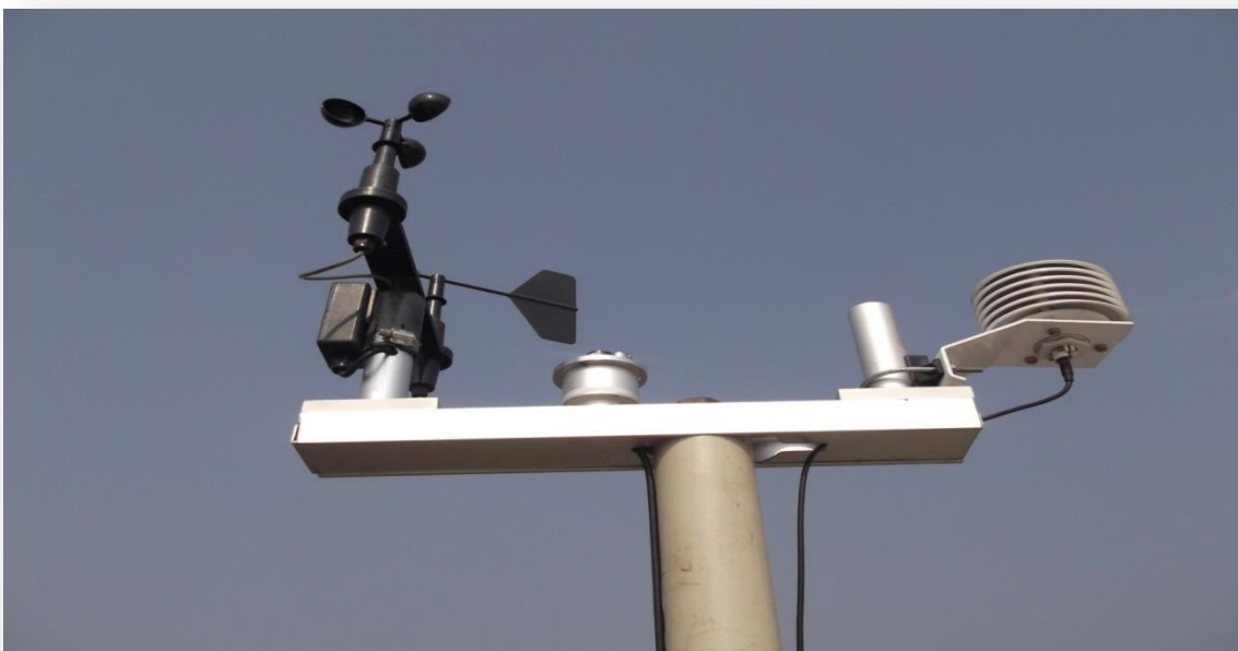
Figure 3: AWS (Automatic Weather Station)
