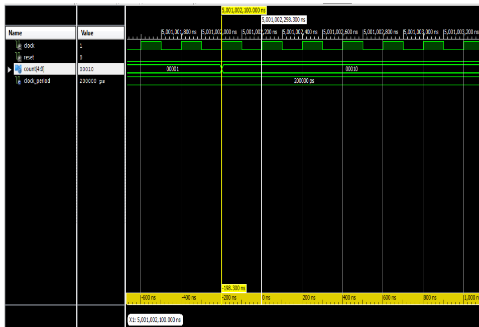
Figure 4: Test bench Behavioural for counter 5-bit
