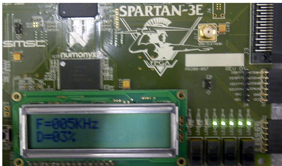
Figure 10: shows the 5 KHz and 3% of duty cycle
