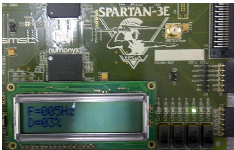
Figure 8: shows the frequency of 5 Hz and the Led for counting
