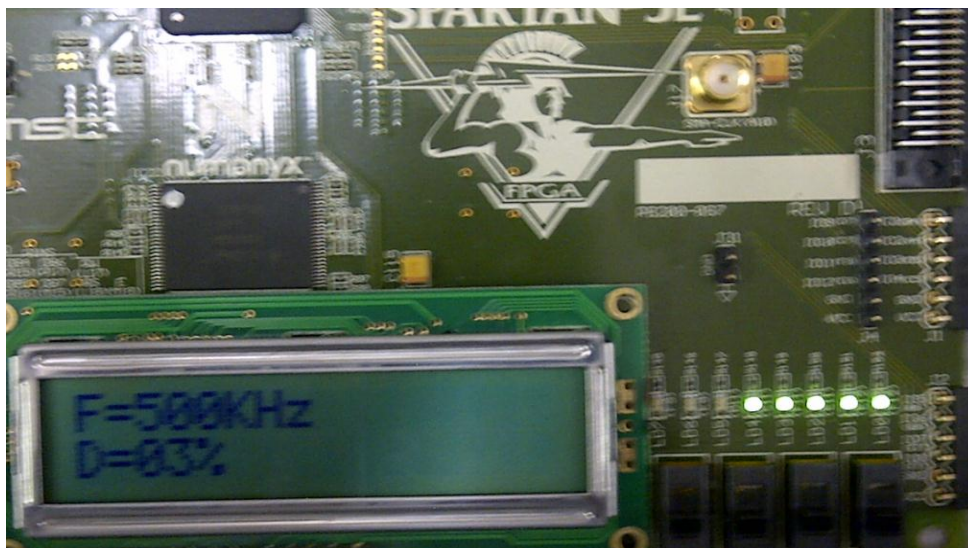
Figure 12: shows the 500 KHz and 3% of duty cycle
