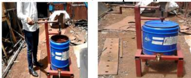
Figure 2. Fabricated Manual Textile chemical mixing and processing machine
