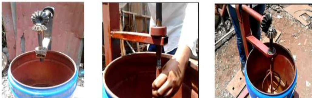
Figure 3. Engaging and removing chemical mixer part (Photo shoot by Author).
