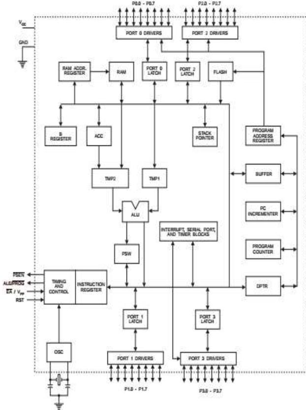
Fig 3: Block Diagram of Micro Controller AT89C52
