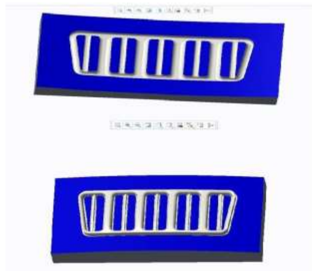
Figure 9. Core and cavity of vertical grille
