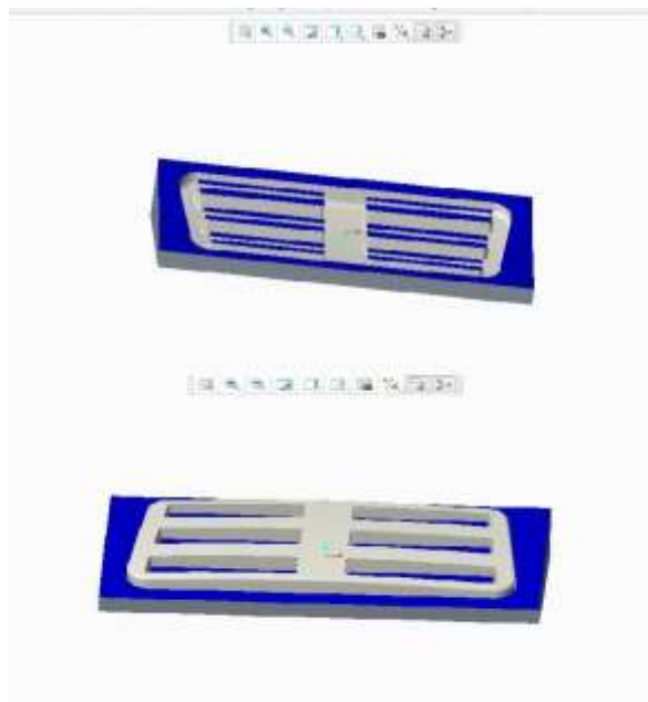
Figure 11. Core and cavity of horizontal grille
