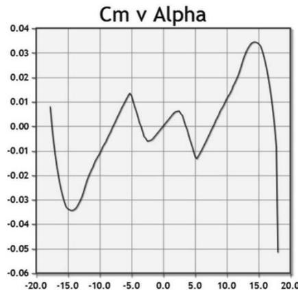
Fig. 11.2. Charts of aerodynamic properties of NACA-0012 at Reynolds no. 500,000.
