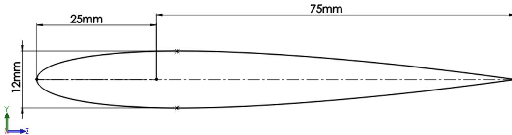
Fig. 11.1. Airfoil NACA-0012.
