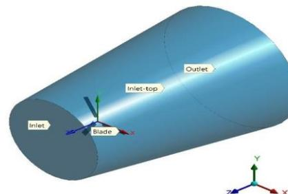
Fig. 12.2. Domain in cylindrical method.
