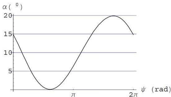
Fig. 10.1. Total effective angle of attack.
