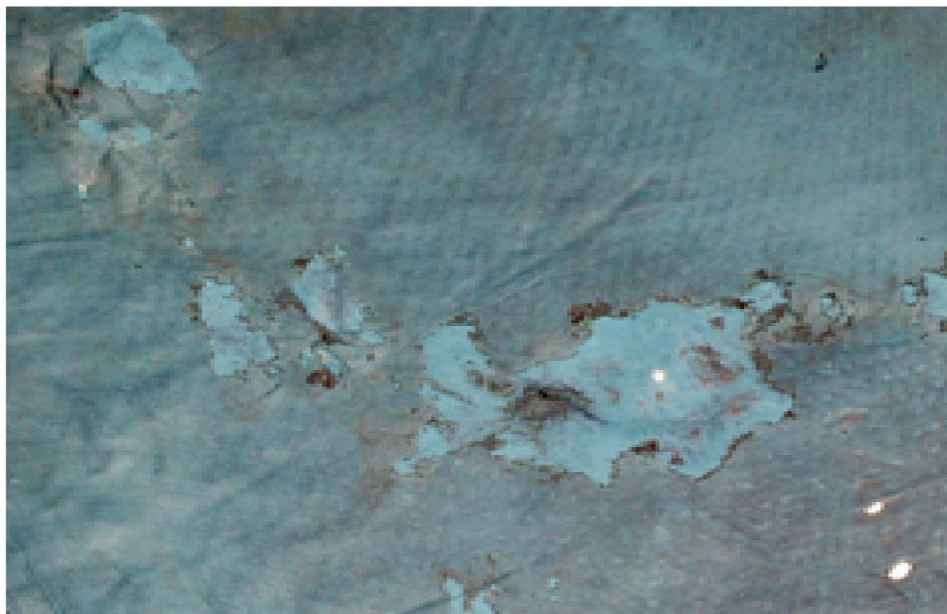
Figure 4. Putrefaction on wet blue cattle hide.
