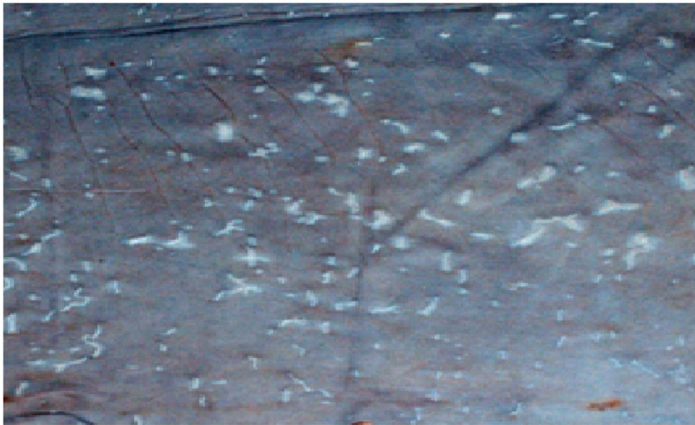
Figure 3. Putrefaction on wet blue sheep skin
