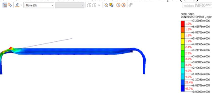
**Figure 13:** Top view of Von Mises stress for Rear Bumper (CPS)
