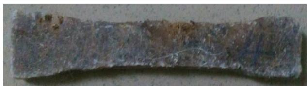
**Figure 4:** Tensile Test specimen [18].
