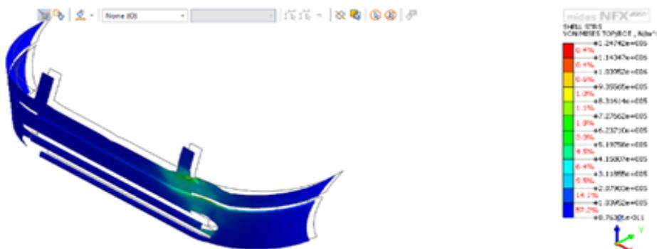
**Figure 7:** Front view of Von Mises stress for Front Bumper (CPS)
