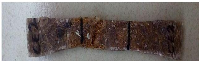
**Figure 5:** Fractured Tensile Test Specimen [18].
