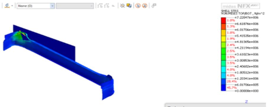
**Figure 12:** Front view of Von Mises stress for Rear Bumper (CPS)
