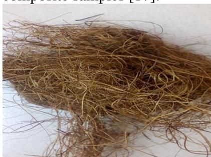
**Figure 1:** Treated coir fiber [17]
