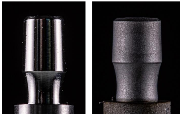
Figure 1. Prosthetic abutment surface before (left side) and after (right side) acid treatment.
