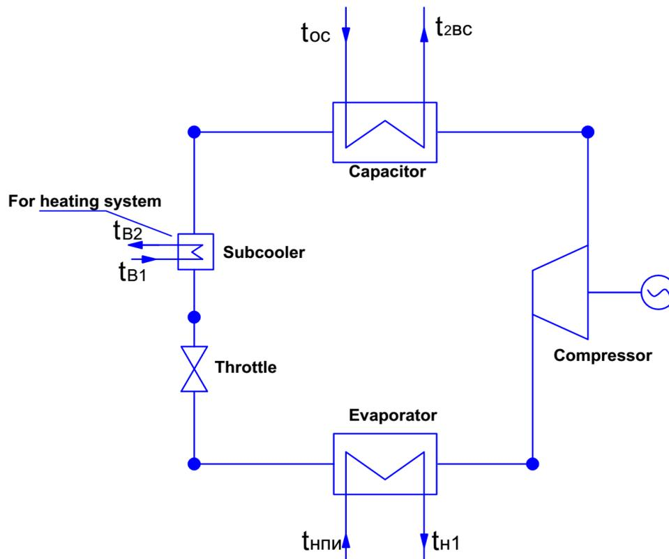
Figure - Schematic diagram of a vapor compression heat pump installation with a pre-cooler
