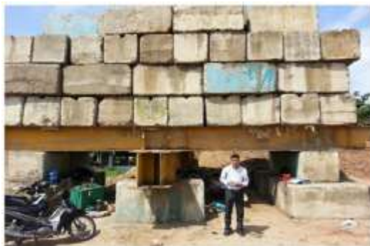
a) Static load test for group SC-pile
