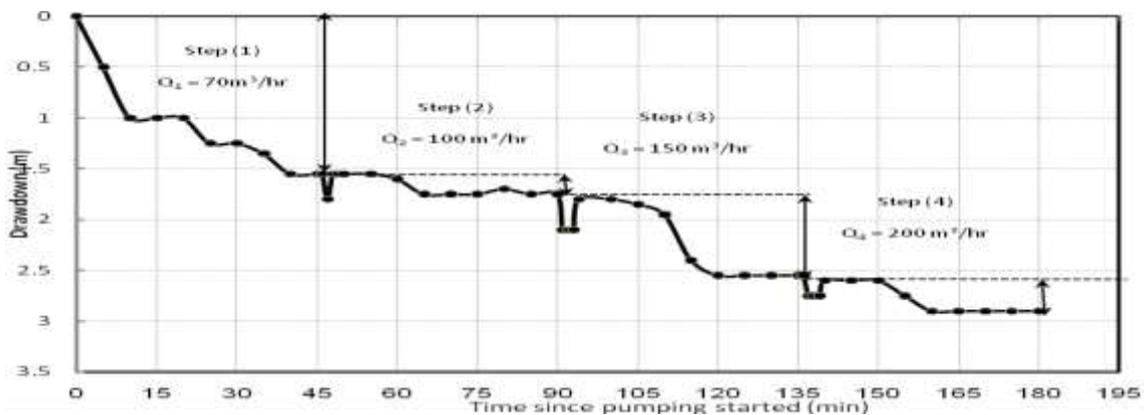
**Figure (9)** Time-Drawdown Data for the Second Step test on March 7, 2011
