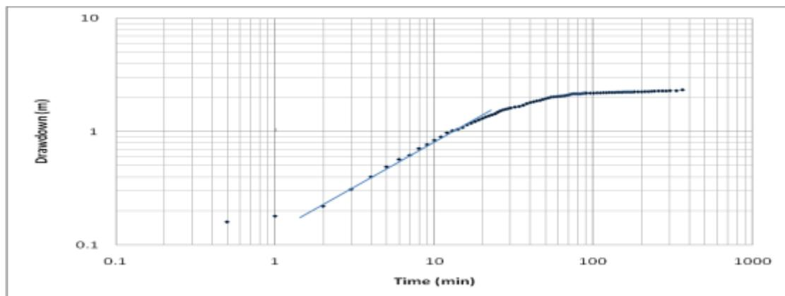
**Figure (16)** Pumping Test Analysis Using Papadopulos-Cooper's Method
