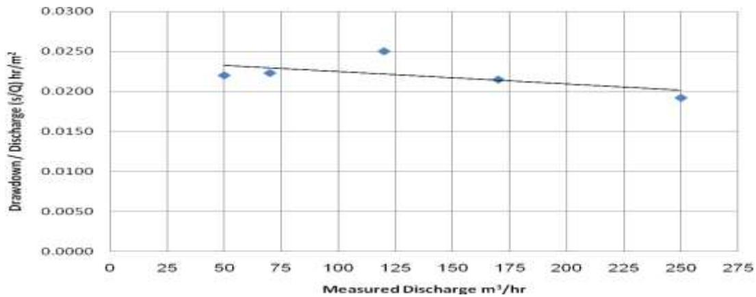
**Figure (12)** Specific Drawdown versus Discharge Rate
