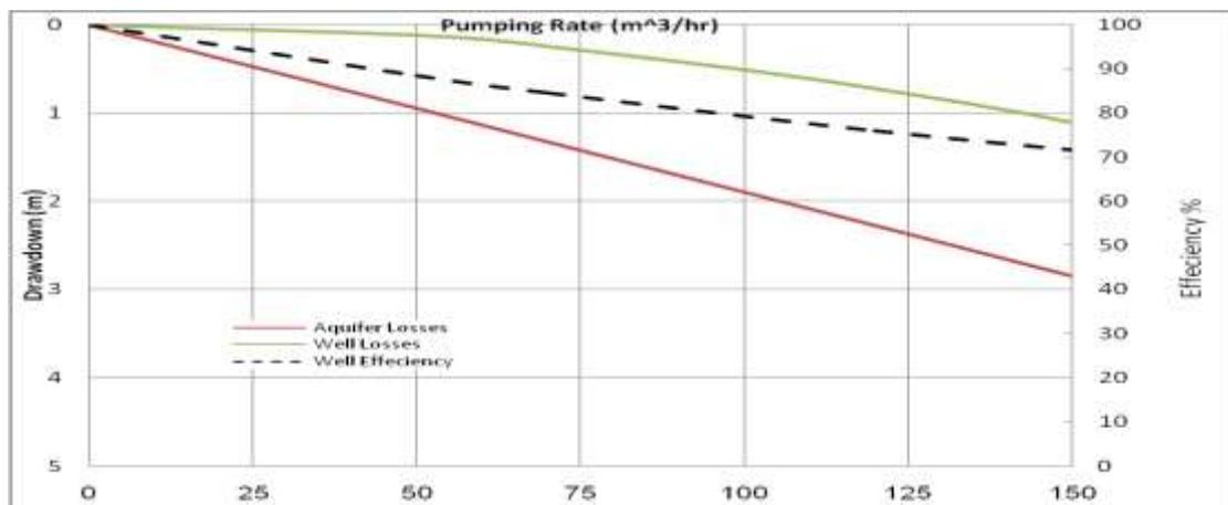
**Figure (14)** Specific Capacity and Efficiency Diagram for the Pumping Well
