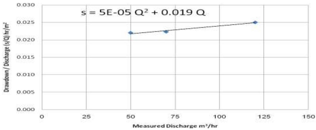
**Figure (13)** Specific Drawdown versus Discharge Rate for the first three stages
