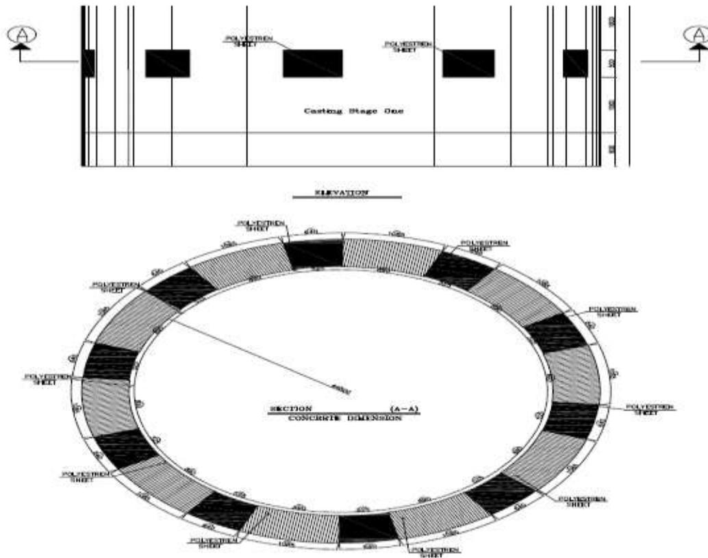
**Figure (5):** Designed Dug Well Elevation and cross section
