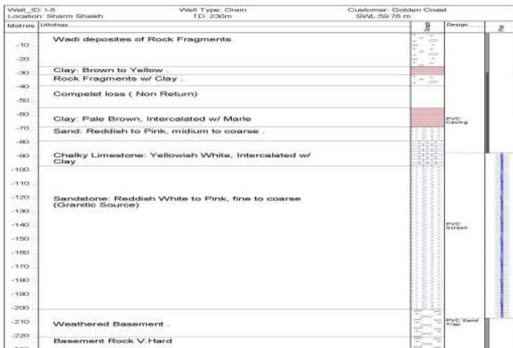
**Figure (3):** Lithologic columnar section of injection well located near the study area
