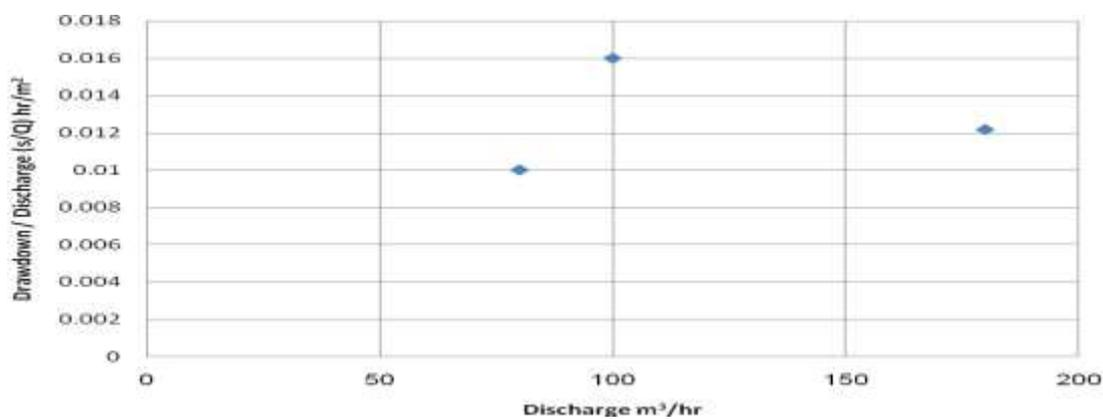
**Figure (8)** Specific Drawdown versus Discharge Rate
