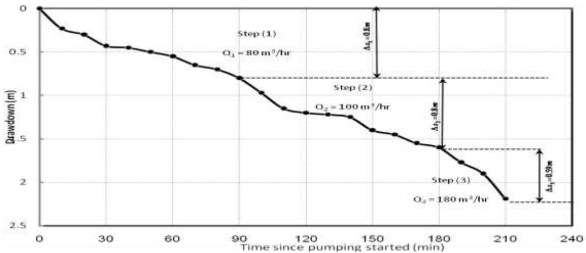
**Figure (7)** Time-Drawdown Data for the First Step test on March 6, 2016
