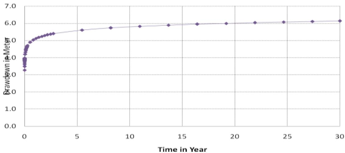
**Figure (17)** Time-Drawdown relationship inside the pumping well
