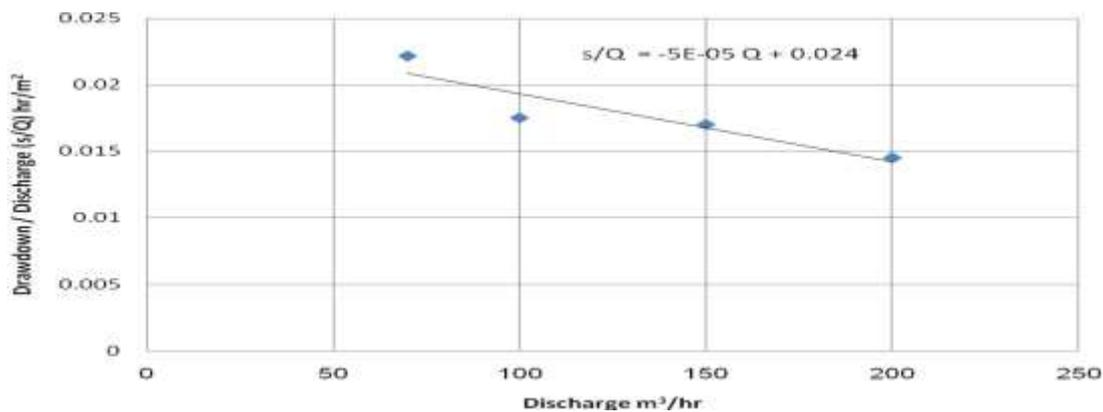
**Figure (10)** Specific Drawdown versus Discharge Rate
