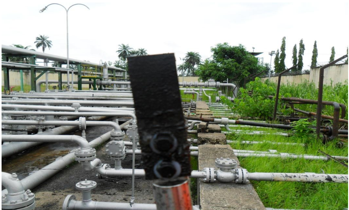
Fig 3: Biofilms on Coupons after 127 days in oil Pipelines
