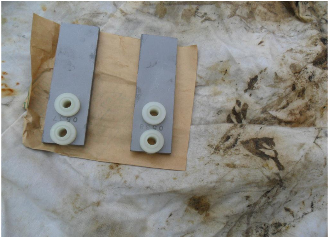
Fig 2: Coupons before insertion into oil Pipelines
