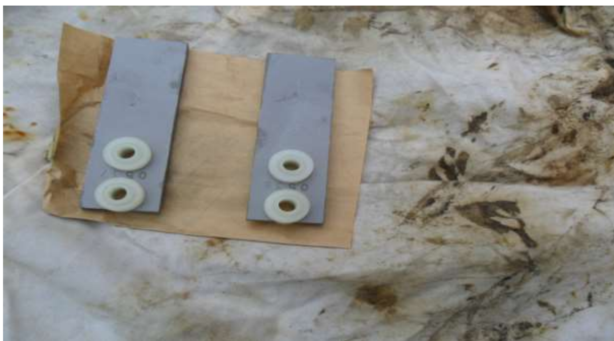
Fig 2: Coupons before insertion into oil Pipelines
