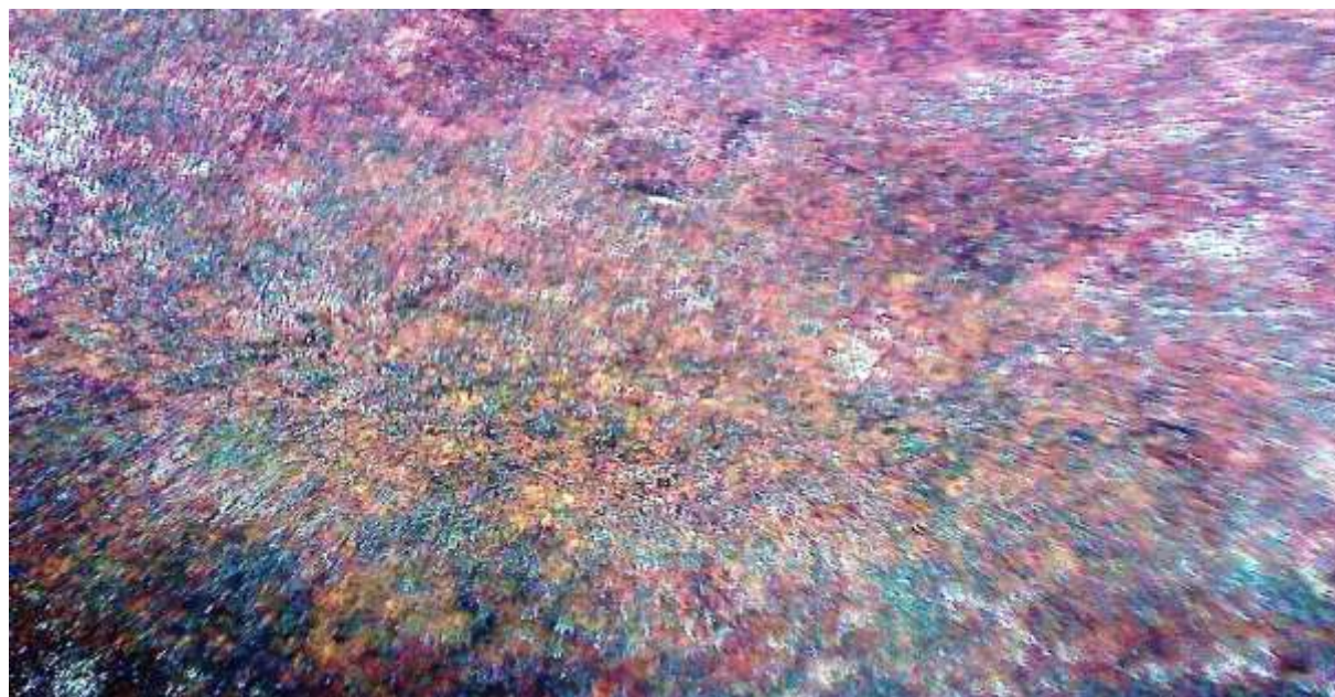
Fig 4: Pit Corrosion on Coupons after 127 days in oil Pipeline
