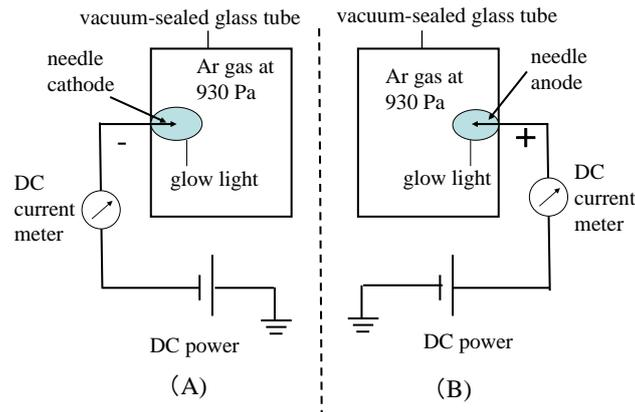
Figure 16 Experimental results of formation of volume of glow lights at around needle electrodes in Ar gas (930 Pa = 7 Torr) in vacuum sealed glass tubes. Needle electrodes respectively have negative potential (A) and positive potential (B) at 2 kV.
