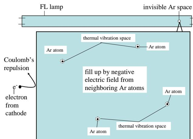
Figure 11 Schematic illustrations that vacuum between Ar atoms fill up negative electric field from orbital electrons in upper shell of Ar atoms. Approaching electrons from cathode of FL lamps cannot get in Ar gas space by strong Coulomb's repulsion.
