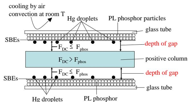
Figure 32 Schematic illustration of cross-section of FL lamp, partially. Electrons only move on in Ar gas space where  $F_{DC} > F_{phos}$ . Commercial phosphor screen is heavily contaminated with insulators; generating deep gap of  $F_{DC} < F_{phos}$ .
