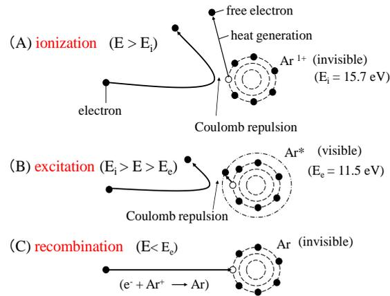
Figure 24 Schematic illustrations of ionization, excitation, and recombination of electron and  $\text{Ar}^{1+}$  by approaching electrons that have different kinetic energy in lighted FL lamps
