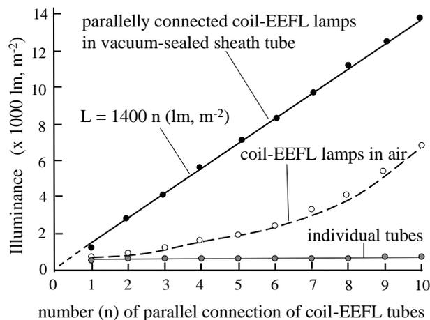
Figure 35 Illuminance ( $\text{lm, m}^{-2}$ ) curves of individual coil-EEFL lamps, coil-EEFL lamps with parallel connection in air, and coil-EEFL lamps in parallel connection in vacuum-sealed sheath tube
