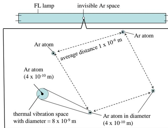
Figure 9 Schematic illustration of distribution of floating Ar atoms in vacuum in FL lamps. Individual Ar atoms in diameter at  $4 \times 10^{-10}$  m isolate each other with distance  $1 \times 10^{-6}$  m. Each Ar atom thermally vibrates in volume of diameter at  $8 \times 10^{-9}$  m.
