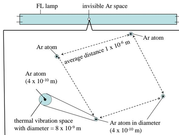
Figure 9 Schematic illustration of distribution of floating Ar atoms in vacuum in FL lamps. Individual Ar atoms in diameter at  $6 \times 10^{-10}$  m isolate each other with distance  $1 \times 10^{-6}$  m. Each Ar atom thermally vibrates in volume of diameter at  $8 \times 10^{-9}$  m.
