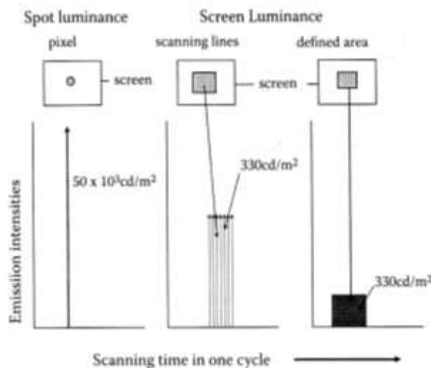
Figure 6 Schematic illustration of same luminance from phosphor screen under different lighting modes under irradiation of electron beam that is a spot, scanning line, and defined area (flame scan)
