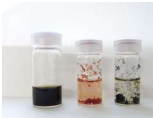
Figure 3. Super-polyphenols can catch the iron(III) ions of the Fe(III)-nta solution, removing the iron(III) ion from the solution
