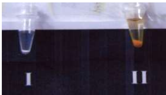
Figure 1. I. Zinc (II) chloride (10 \mu\text{L} , 1 M) was added to the A \beta (1-40) solution (100 \mu\text{L} , 0.25mg/ mL). II. \text{Fe}_2(\text{HPTP})\text{Cl}_4\text{ClO}_4 solution (50 \mu\text{L} , 2 mg/mL) was added to the solution I . Brown precipitates occurred immediately upon the addition of \text{Fe}_2(\text{HPTP})\text{Cl}_4\text{ClO}_4 solution.
