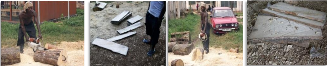
Plate 34 Cutting of Log into Boards
