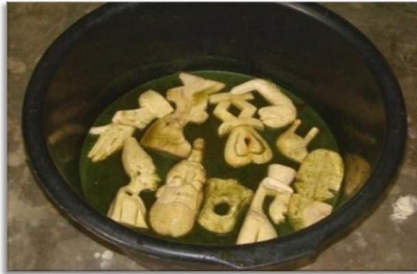
Plate 26 Freshly carved objects in liquid substance for treatment.
