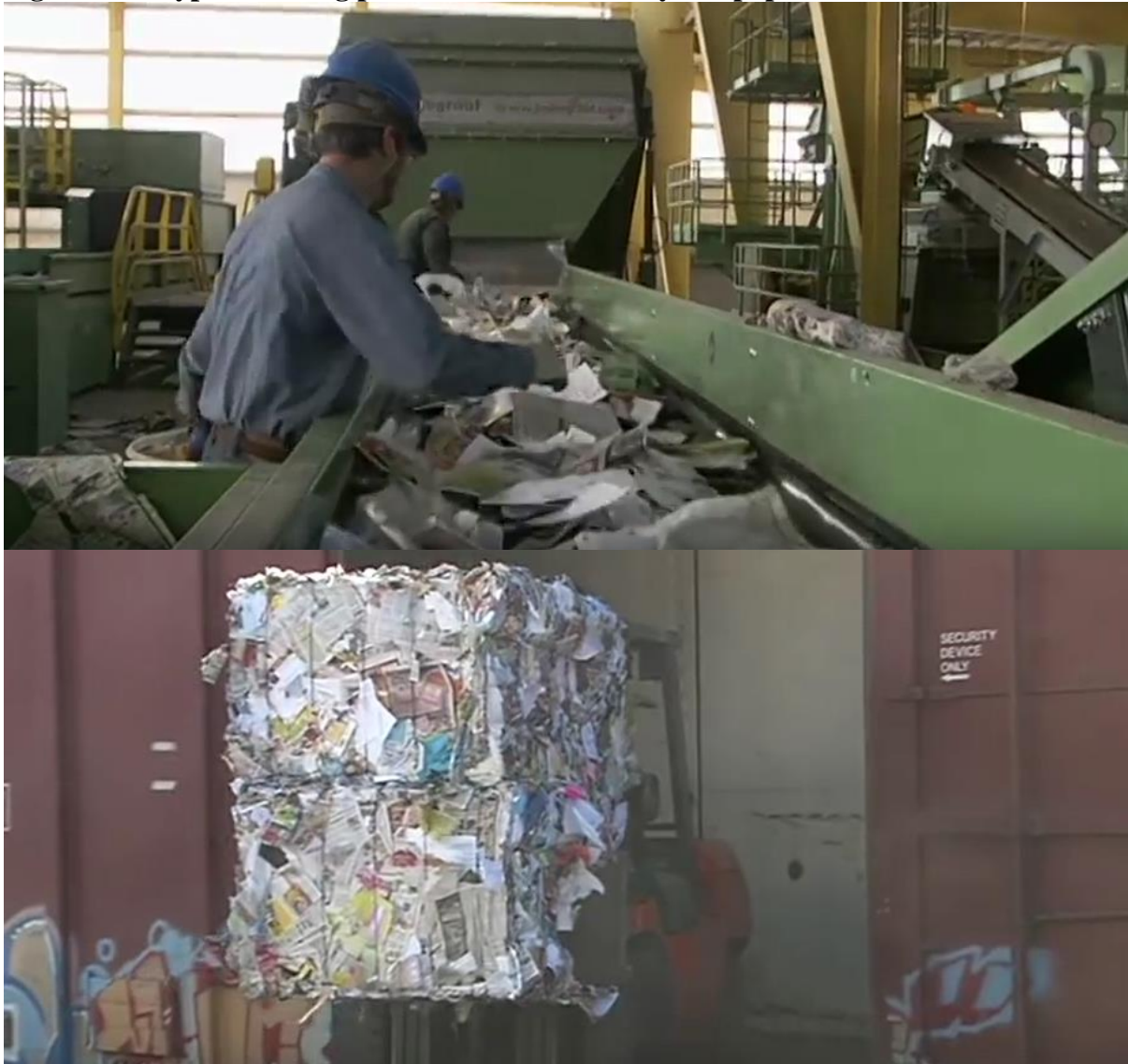
Figure 12 – Typical sorting process and bales of recycled paper
