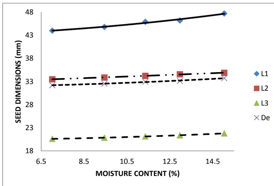
**Fig. 3.1 Effect of moisture content on seed dimensions**
