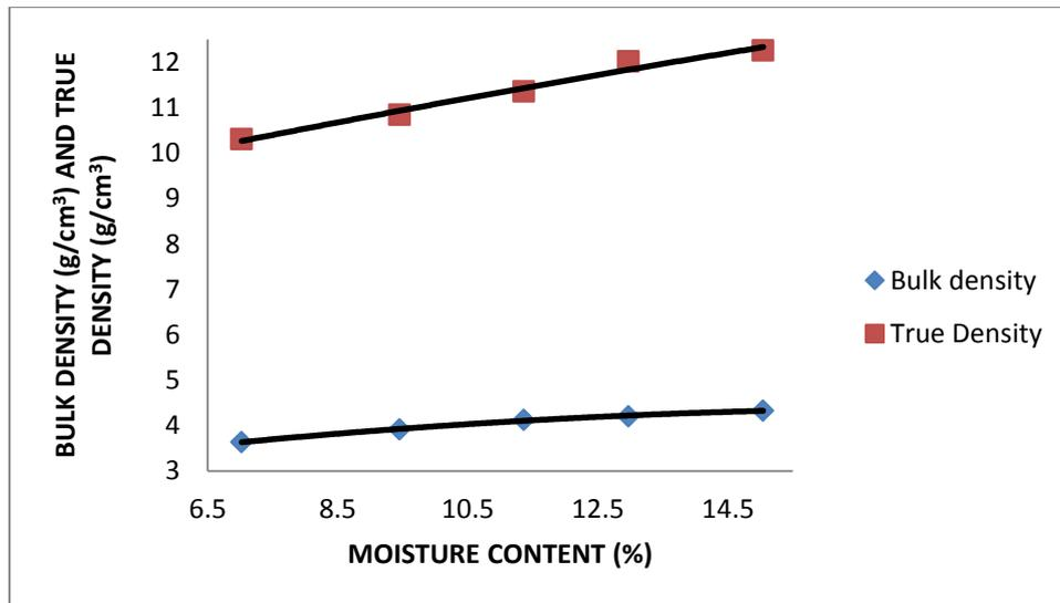
**Fig. 3.3 Effect of moisture content on densities**
