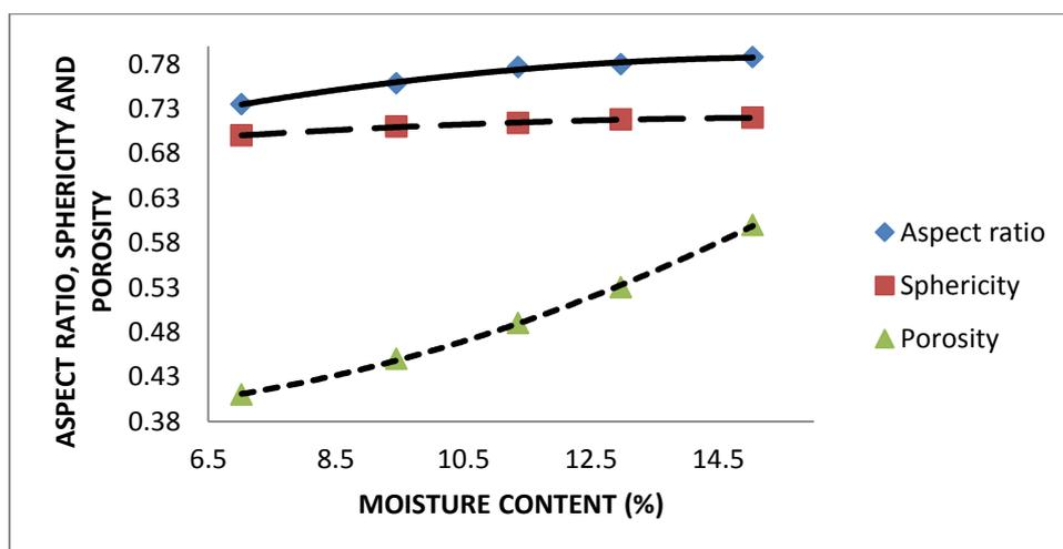
**Fig. 3.4 Effect of moisture content on aspect ratio, sphericity and porosity**
