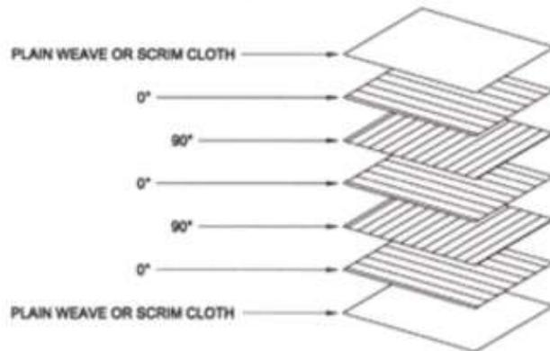
Figure 9: Schematics of the fiber layers for one half of the bi-directional CFRP model. The impact velocities on CFRP were 0.6 km/s, 0.8 km/s and 1 km/s. A capture of the impact is presented in *Figure 10*.
