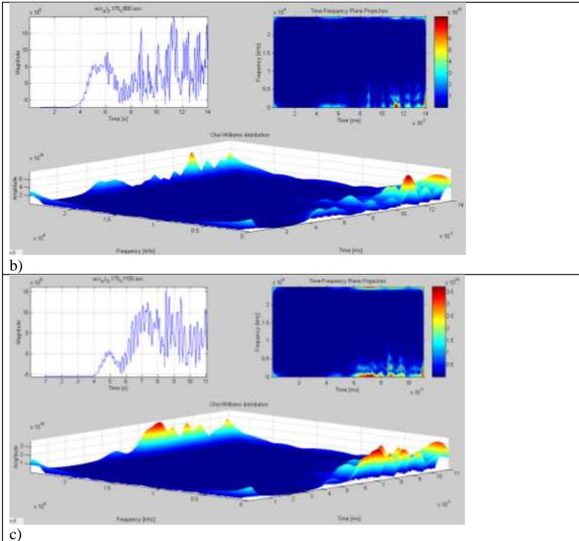
Figure 6: CWD for impact on Al6061-T6 of 0.3175 cm thickness: a) non-penetration; b) penetration limit; c) full penetration.
