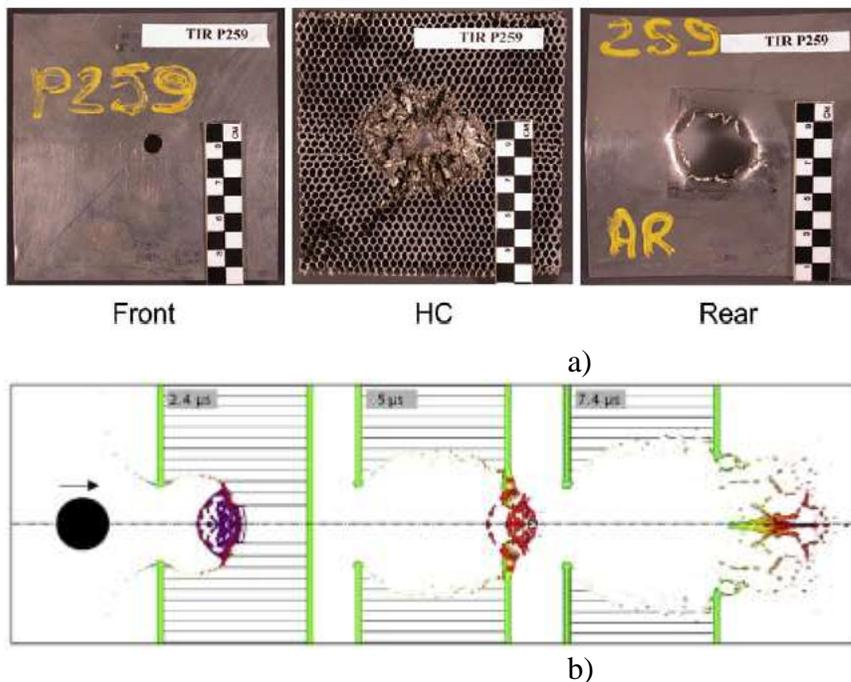
Figure 1: Channelling effect created in an HC/SP impacted at 5.7 Km/s; a) test samples, b) simulation (13)
