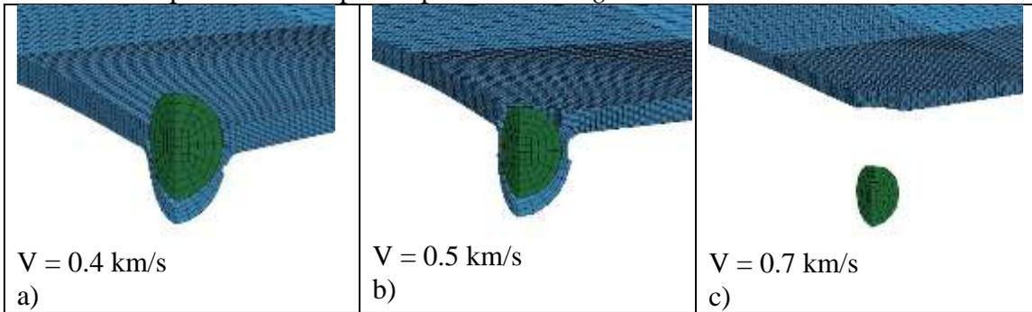
Figure 7: Impact simulation on Ti plate of 0.08128 cm thickness: a) non-penetration; b) penetration occur/penetration limit; c) full penetration.
