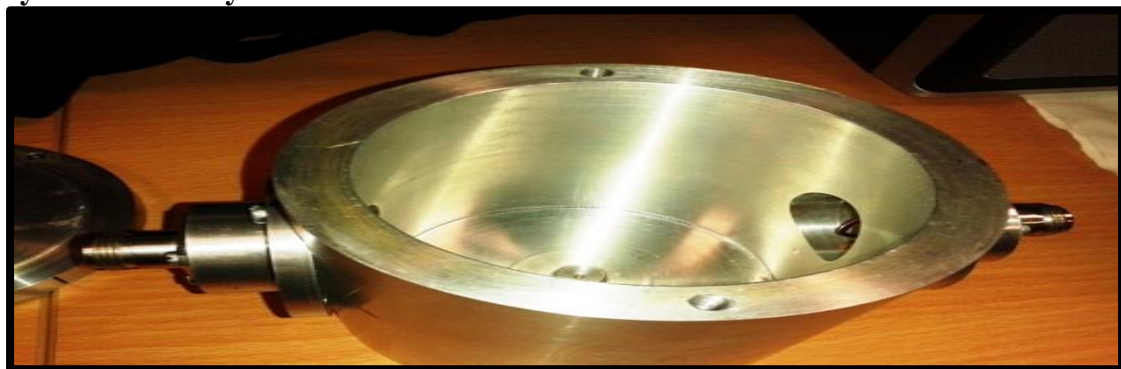
Figure 2: Ports 1 & 2 with loop antenna at each one inside the cavity.
