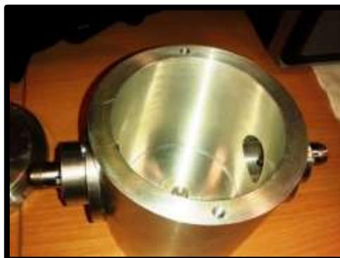
**Figure 2: Ports 1 & 2 with loop antenna at each one inside the cavity.**
