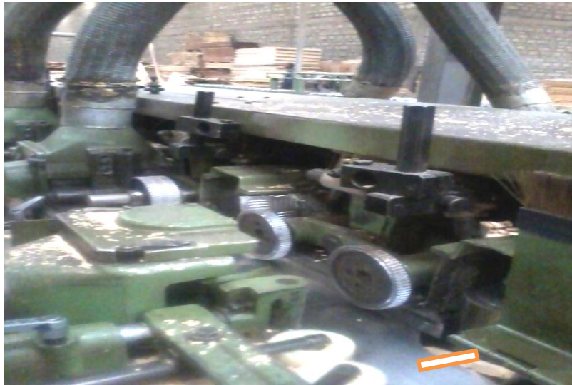
Plate 2: Unguarded machines at RaiPly wood industry in Eldoret Municipality, Kenya
