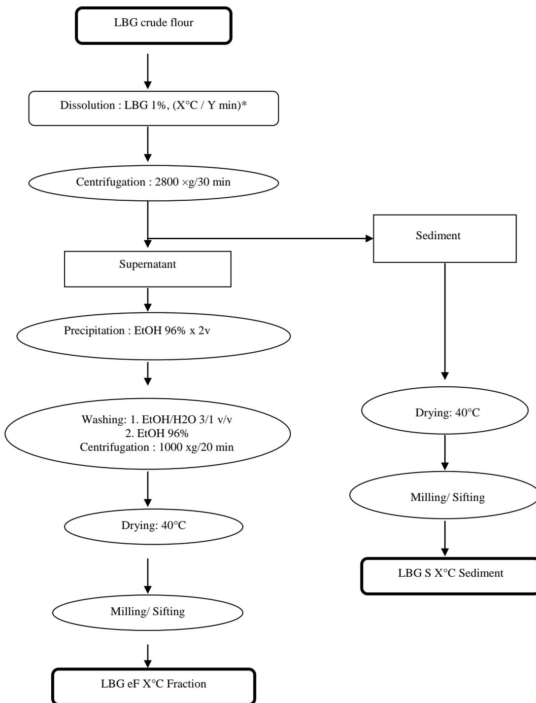
**Fig. 2: Process of carob gum flour simple fractionation at different temperature. \*(at 23°C/60 min, 37°C/45 min, or 80°C/30 min).**
