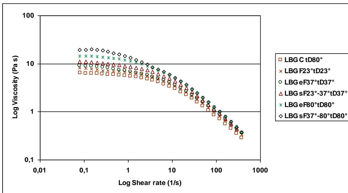
**Fig.5. Viscosity curves rheograms of all extracted LBG samples and crude gum (LBG C) measured at 25°C, 1% concentration. tD= Dissolution temperature.**
