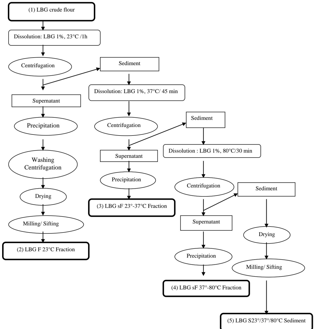
**Fig. 1: Process of carob gum flour sequential (subtractive) fractionation by temperature of solubilisation**
