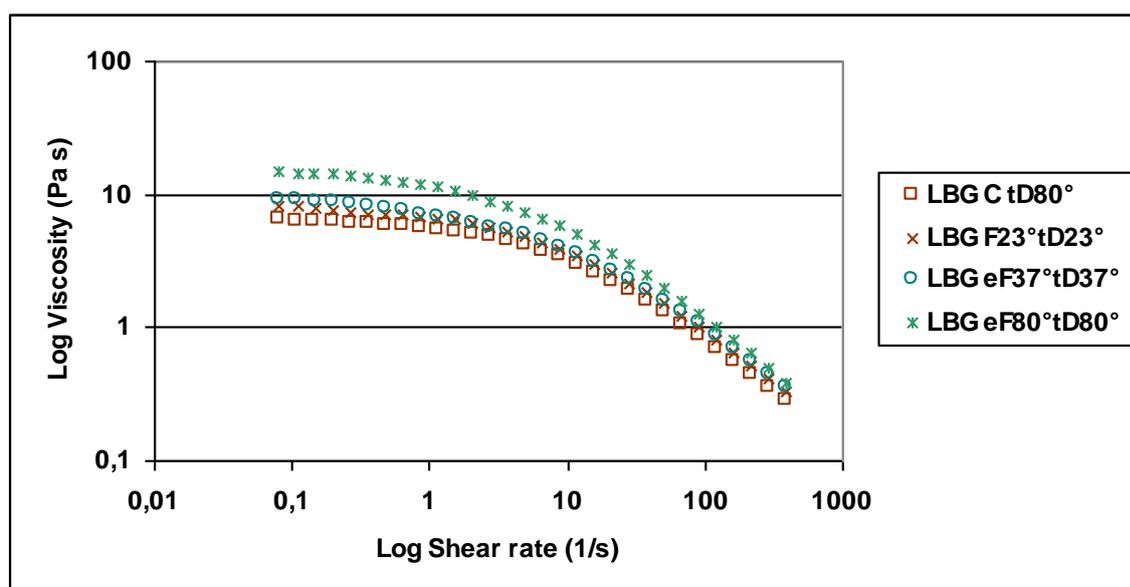
**Fig.4. Plot of apparent viscosity behaviour vs. Shear rate for entire purified fractions (LBG eF) and crude (LBG C) of Locust bean gum measured at 25°C, 1% concentration. tD= Dissolution temperature.**
