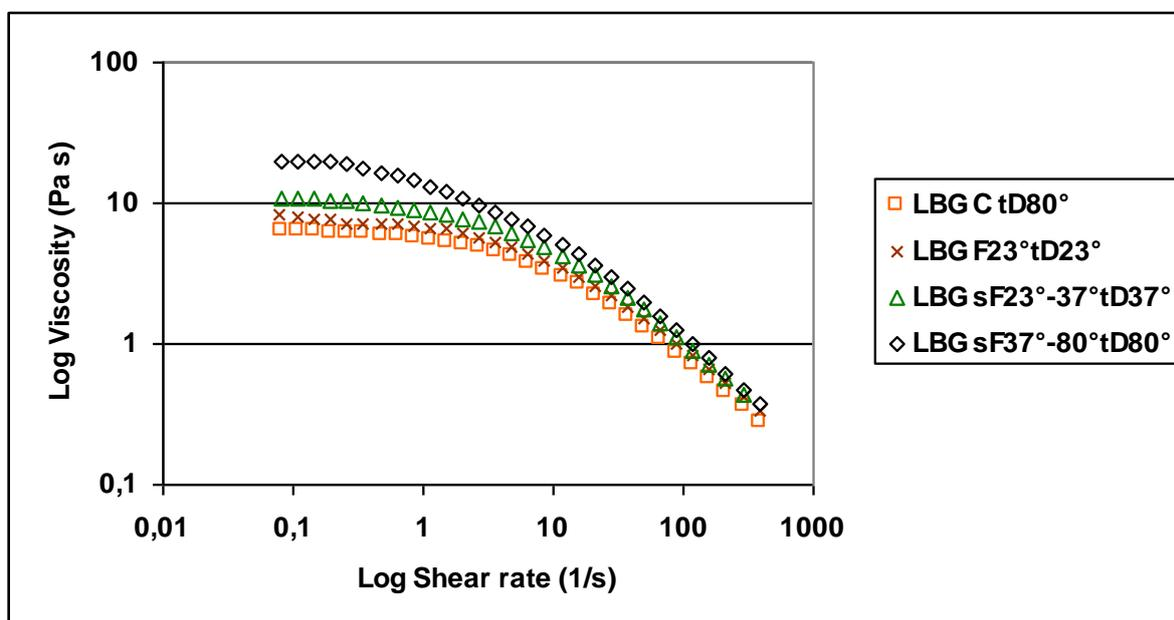
**Fig.3. Plot of apparent viscosity behaviour vs. Shear rate for sequential purified fractions (LBG sF) and crude (LBG C) of Locust bean gum measured at 23°C, 1% concentration. tD= Dissolution temperature.**
