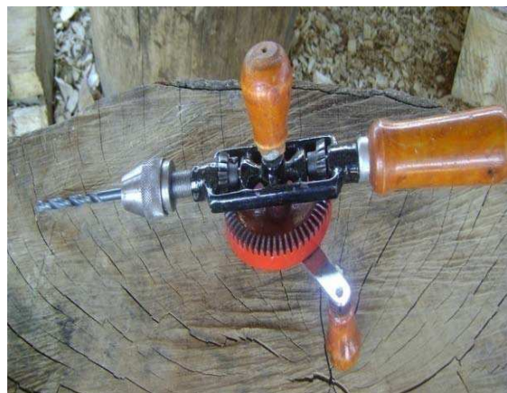
Plate 9 – Hand Drill: for drilling holes in the carvings
