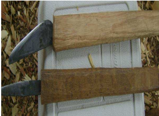
Plate 3 – Knives (sekenmoa) – used to for clearing Pare, cut and smoothen wood.
