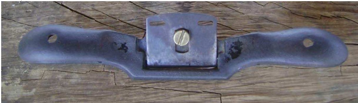
Plate 7 - Spoke shave: Is used to shape and smooth convex and concave wooden surfaces
