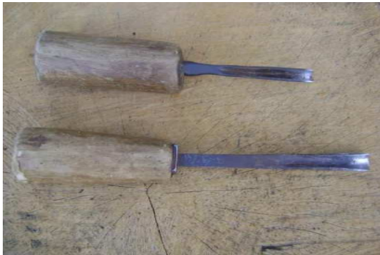
Plate 5 – 'V' Gouge: Is a 'V' shaped cutting cutting deep and edge used for parting, outlining or emphasizing round curves and for boring holes, lines and decorative cuts.
