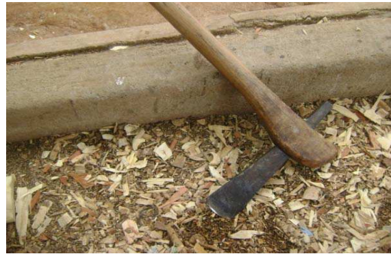
Plate 1 – Adze (soso): used for carving handle and heavy metal used for chopping wood.
