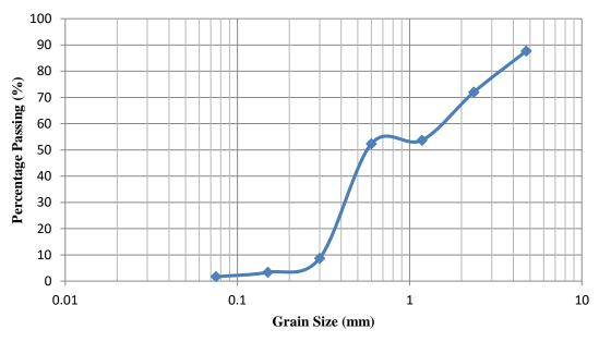
FIGURE 4: Grain size distribution curve
