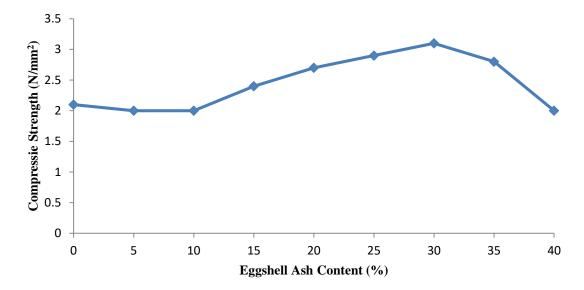
Figure 5: Variation of compressive strength of sandcrete block at varying eggshell ash content for 7 days curing period
