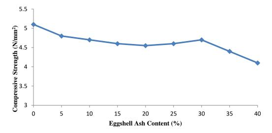
Figure 8: Variation of compressive strength of sandcrete block at varying eggshell ash content for 28 days curing period
