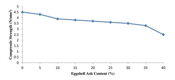
Figure 6: Variation of compressive strength of sandcrete block at varying eggshell ash content for 14 days curing period
