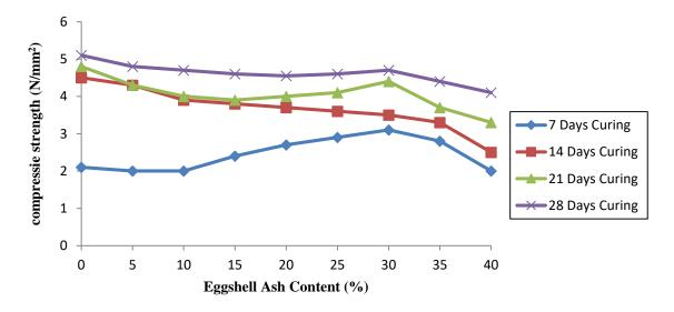
Figure 9: Variation of compressive strength of sandcrate block with eggshell ash content at varying curing period in days
