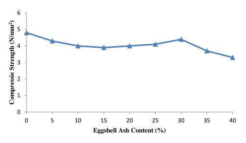
Figure 7: Variation of compressive strength of sandcrete block at varying eggshell ash content for 21 days curing period
