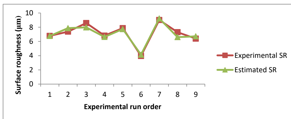
Figure 3: Comparison between measured and predicted value for surface roughness of Mild Steel
