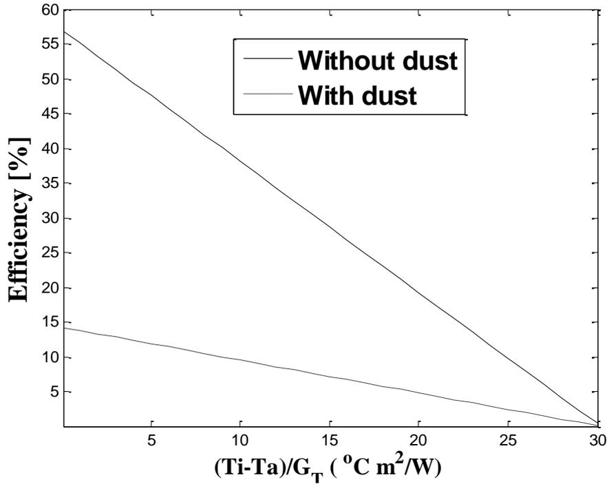
**Figure 4: Dust effect on the relationship between thermal efficiency and the  $(T_i - T_a)/G_T$**
