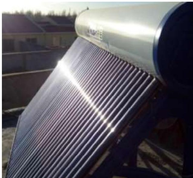
**Figure 1: Evacuated Tube Collectors Used for Experiments**
