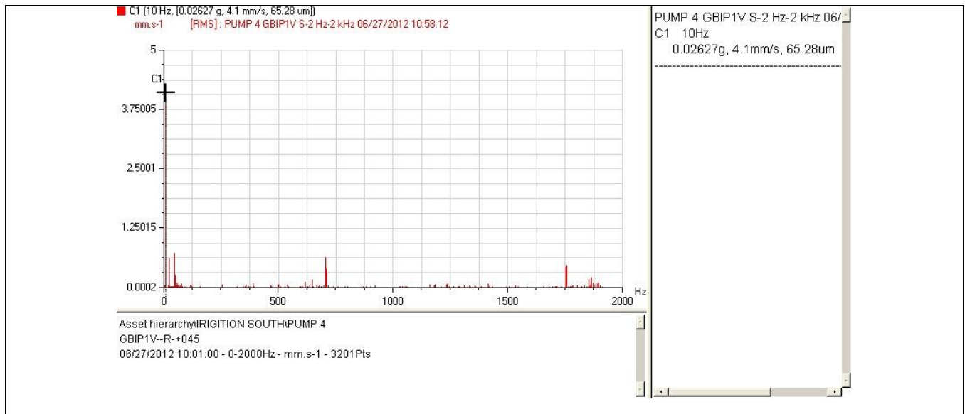
(c) Gear Box pump side horizontal
