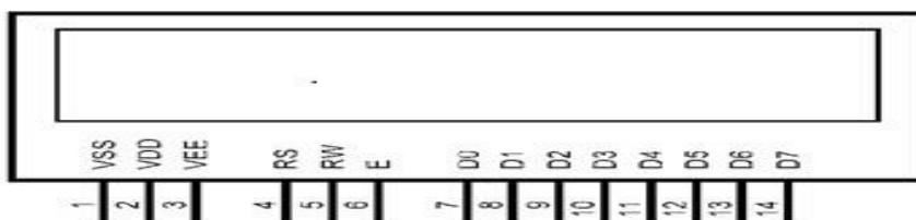
Figure 8: Pin configuration of the 16x2 matrix LCD
