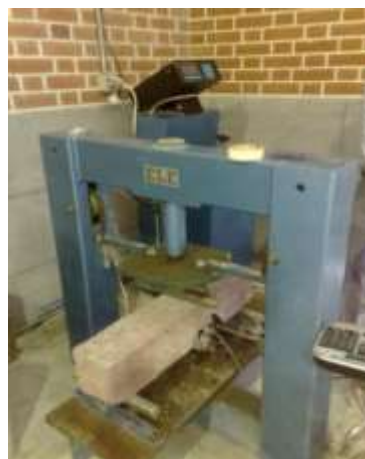
Fig. 4. Test setup for Flexural Strength
