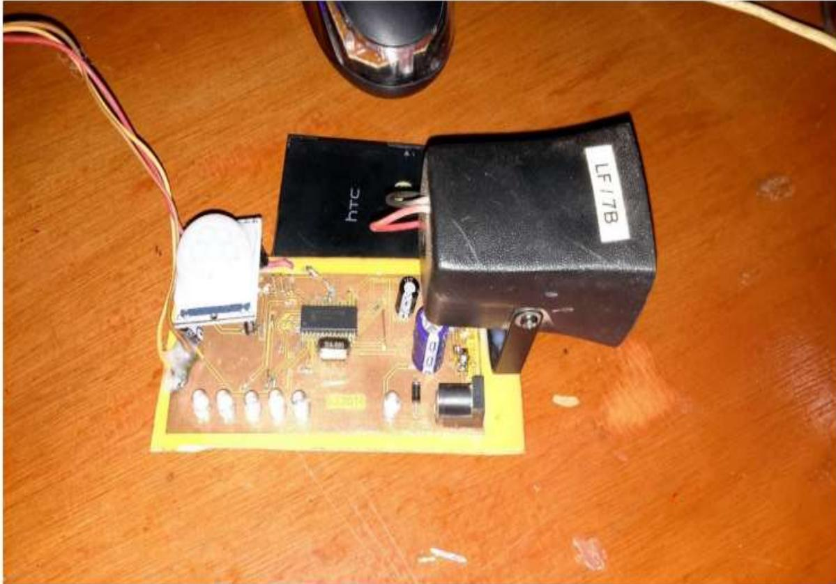
**Fig. 10: The completed work with the PIR motion Sensor and siren speaker system under test.**
