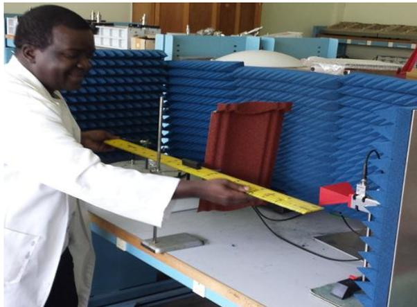
**Figure 7. Measurement of transmission distance**
