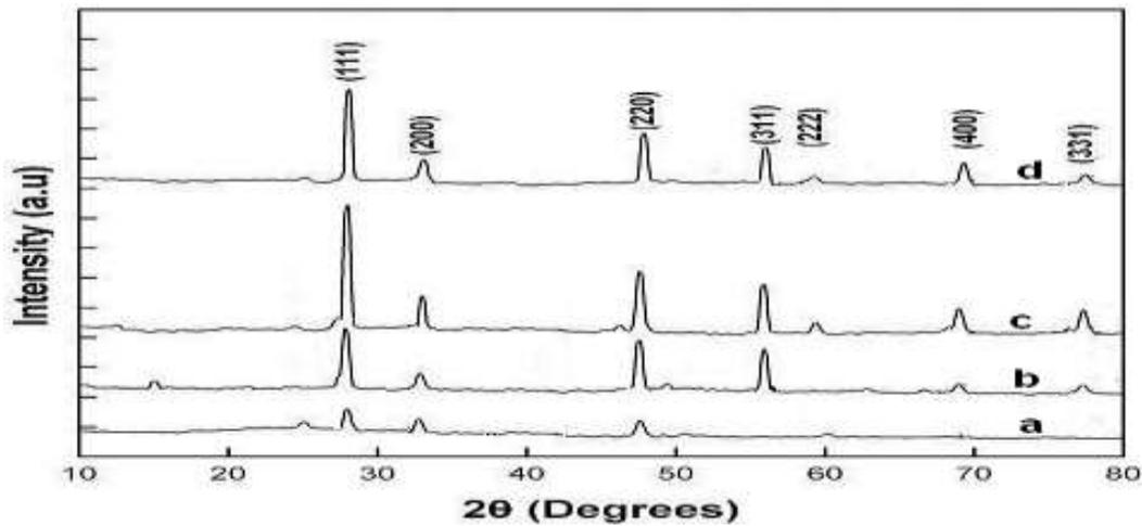
Figure 2 :XRD of  $(\text{CuS})_x(\text{Fe})_{(1-x)}$  composite thin films: (a)  $(\text{CuS})_{0.50}(\text{Fe})_{0.50}$  (b)  $(\text{CuS})_{0.20}(\text{Fe})_{0.80}$ , (c)  $(\text{CuS})_{0.1}(\text{Fe})_{0.9}$ , (D) CuS
