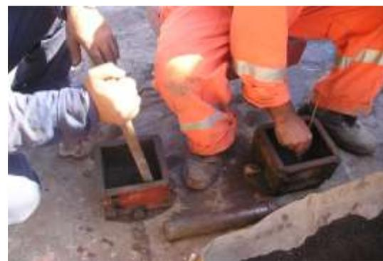
Prepare cube and compaction of concrete mix
