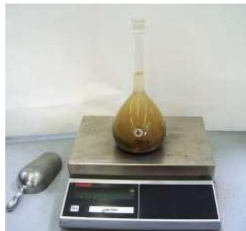
Fig.7 Specific gravity testing
