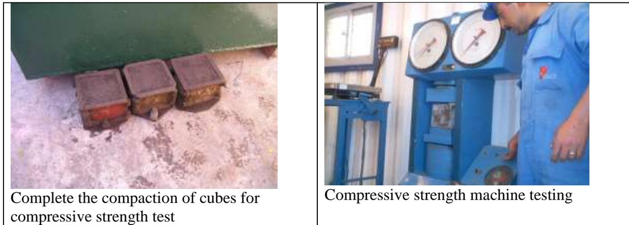
**Fig. 9: Concrete mix of hematite- barite ore aggregate, Sea water cement & fresh water ( 15\*15\*15 cm )**
