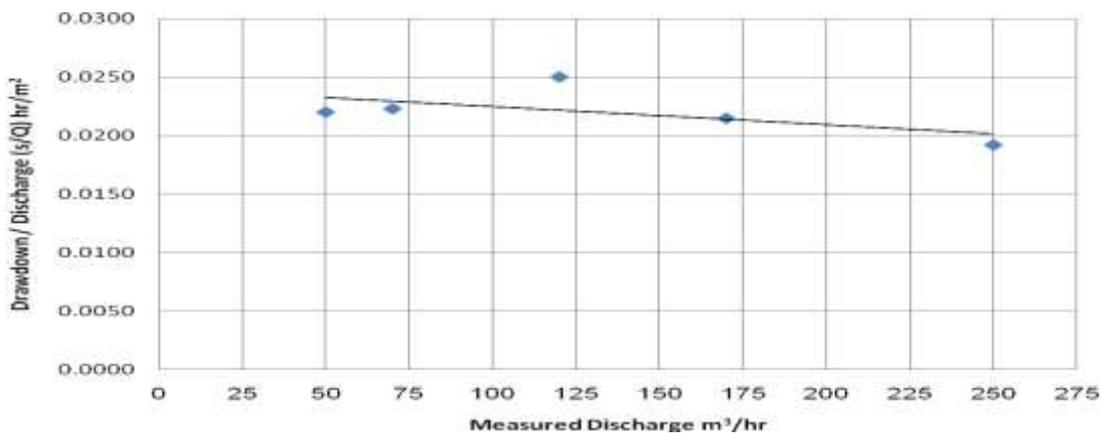
**Figure (12)** Specific Drawdown versus Discharge Rate
