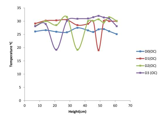
Figure 1.0: A graph of Temperature Distribution against Height for Four Non-Convective Pools at 7am,  $T_a = 24.9^{\circ}$ C on Nov. 22, 2012
