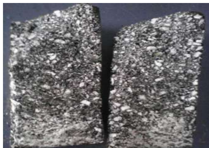
Figure 09: Failure of M21 Concrete cylinder
