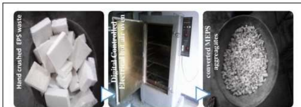
Figure No. 01: Processing of Waste EPS by heat treatment
