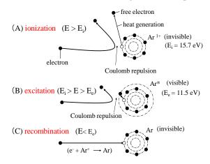
Figure 24 Schematic illustrations of ionization, excitation, and recombination of electron and  $Ar^{1+}$  by approaching electrons that have different kinetic energy in lighted FL lamps
