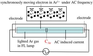
Figure 15 Formation mechanism of capacitor CAr in lighted FL lamp
