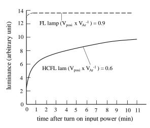
Figure 34 Build-up curves of light of FL lamp having  $(V_{posi} \times V_{Ar}^{-1}) = 0.8$  and Commercial HCFL lamp that has  $(V_{posi} \times V_{Ar}^{-1}) = 0.6$
