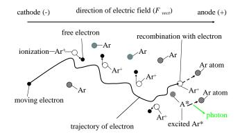
Figure 26 Schematic illustration of moving trajectory of given electron in superconductive vacuum, generating many  $Ar^{1+}$ , one  $Ar^*$  and then return to Ar atom.
