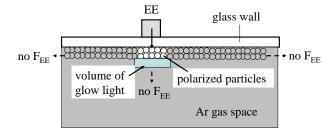
Figure 31 Illustration of polarized phosphor particles in screen by electric field from external electrode and formation of volume of glow lights as internal cathode (or anode) in Ar gas space
