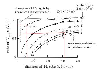
Figure 33 Curves of  $(V_{posi} \times V_{Ar}^{-1})$  of FL lamps as a function of outer diameters of FL lamps. Parameter is depth of gap in FL lamps
