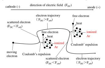
Figure 25 Schematic explanation of moving electron under electric field  $F_{DC}$  and change of trajectory by Coulomb's repulsion from two Ar atoms. Each Coulomb's repulsion generates  $Ar^{1+}$  and free electron in Ar gas space
