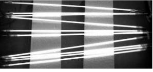
(A) 10 parallel connection of coil-EEFL lamps under DC 3kV
