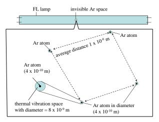
Figure 9 Schematic illustration of distribution of floating Ar atoms in vacuum in FL lamps. Individual Ar atoms in diameter at  $6 \ge 10^{-10}$  m isolate each other with distance  $1 \ge 10^{-6}$  m. Each Ar atom thermally vibrates in volume of diameter at  $8 \ge 10^{-9}$  m.
