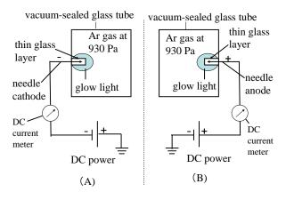
Figure 20 Illustration of volume of glow light on thin glass layer on needle electrodes. Experiments are made with the DC voltage at 2 kV
