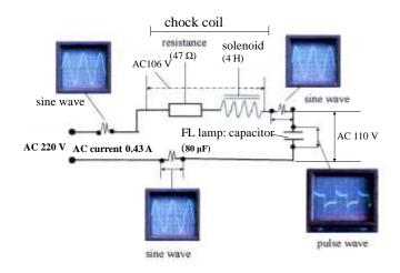
Figure 13 AC driving circuit (ballast) of 40W-HCFL lamp with waveforms at components
