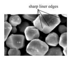
Figure 27 Photograph of phosphor particles under scanning electron microscope (x 3000)
