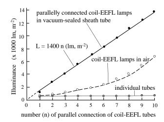
Figure 35 Illuminance (lm, m<sup>-2</sup>) curves of individual coil-EEFL lamps, coil-EEFL lamps with parallel connection in air, and coil-EEFL lamps in parallel connection in vacuum-sealed sheath tube
