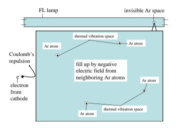
Figure 11 Schematic illustrations that vacuum between Ar atoms fill up negative electric field from orbital electrons in upper shell of Ar atoms. Approaching electrons from cathode of FL lamps cannot get in Ar gas space by strong Coulomb's repulsion.
